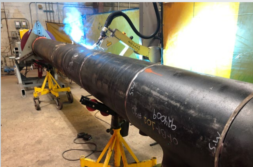
Spool welding robot SWR in action at a shipyard
