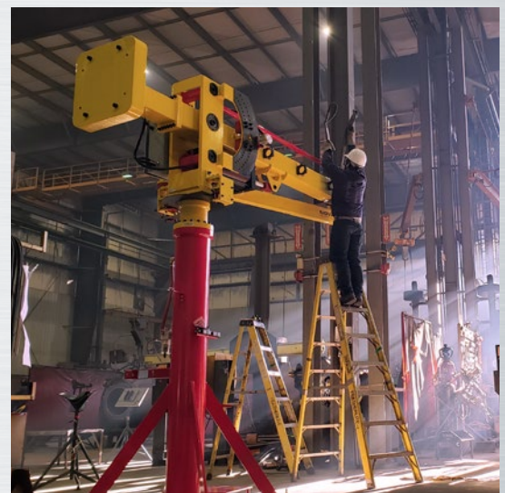
Construction of the spool welding robot SWR at one of the largest planning, procurement and construction companies in Edmonton, Canada
